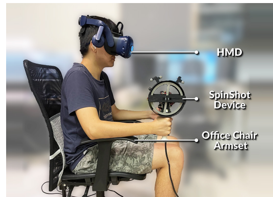
Figure 10: Study setup with a participant sitting in a chair with the dominant arm supported while holding the device.
